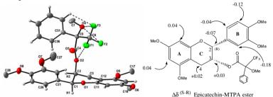
The crystal structure of (-)-epicatechin-(R)-MTPA is described and the origin of the conformational behaviour observed for MTPA esters is explained.
